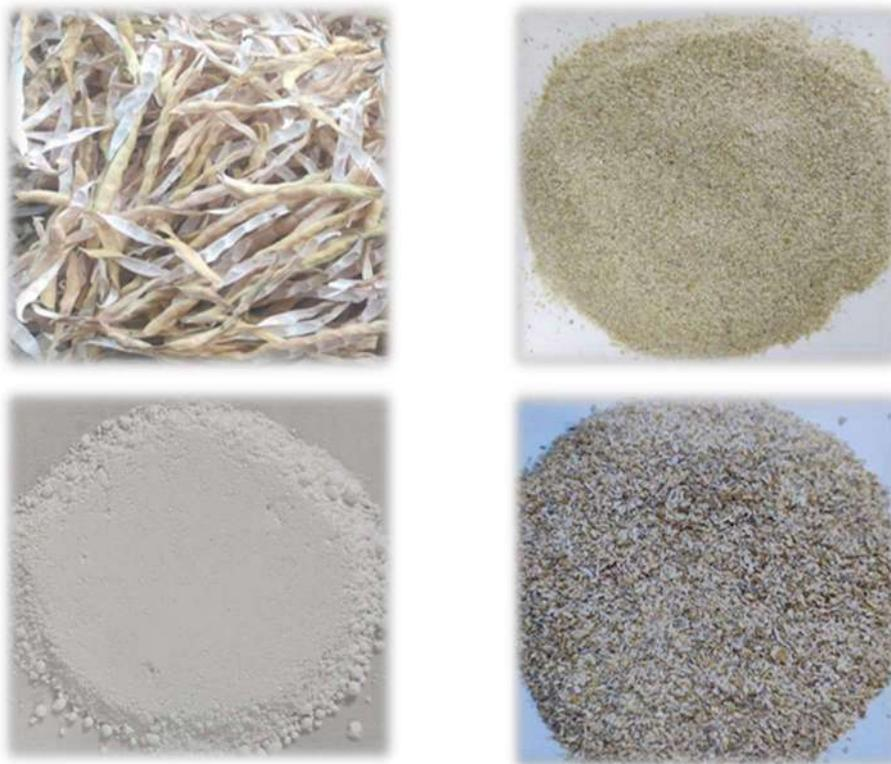
**Fig (1) : The cowpea husk collection(a), The cowpea husk ground(b), ZnO nanoparticles(c), The cowpea husk after coating with ZnO nanoparticles(d)**
