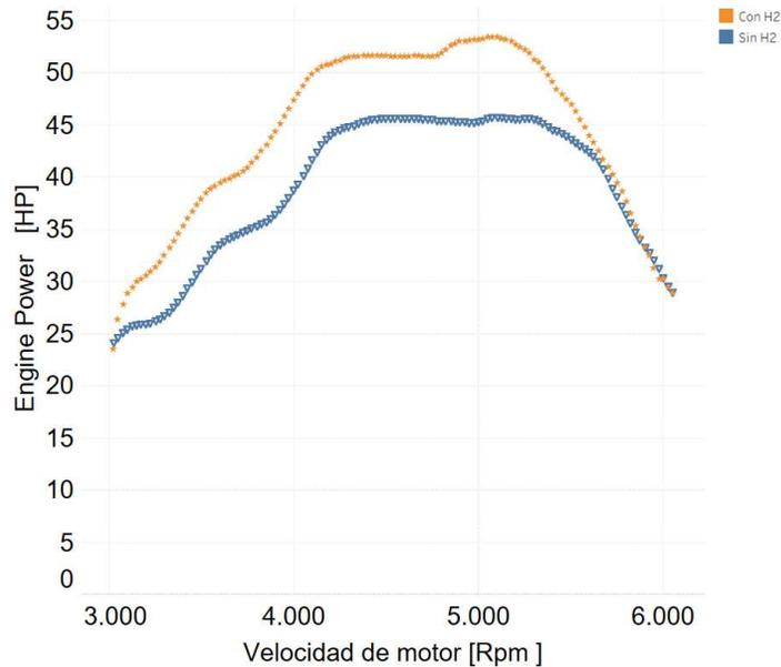
Figure 4 Power comparison with H2 and without H2
