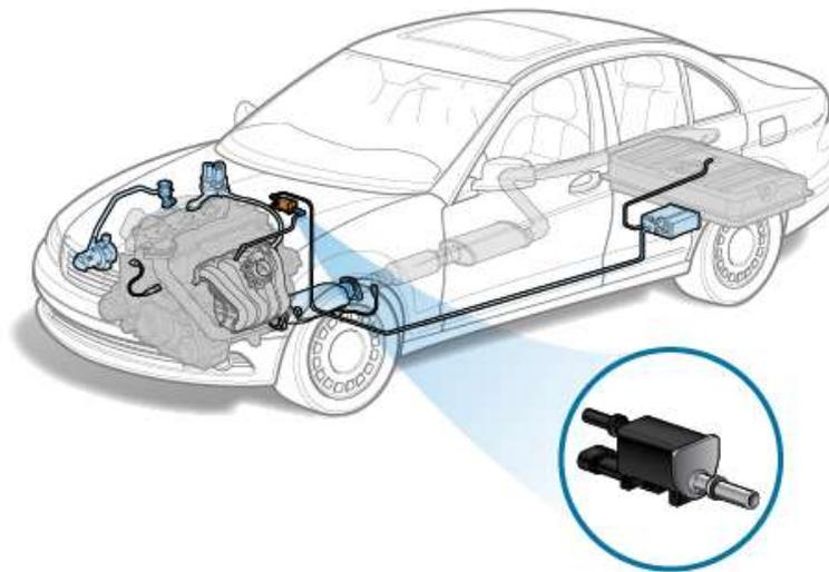
Figure 2. Location of the hydrogen injection valve to the internal combustion engine.
