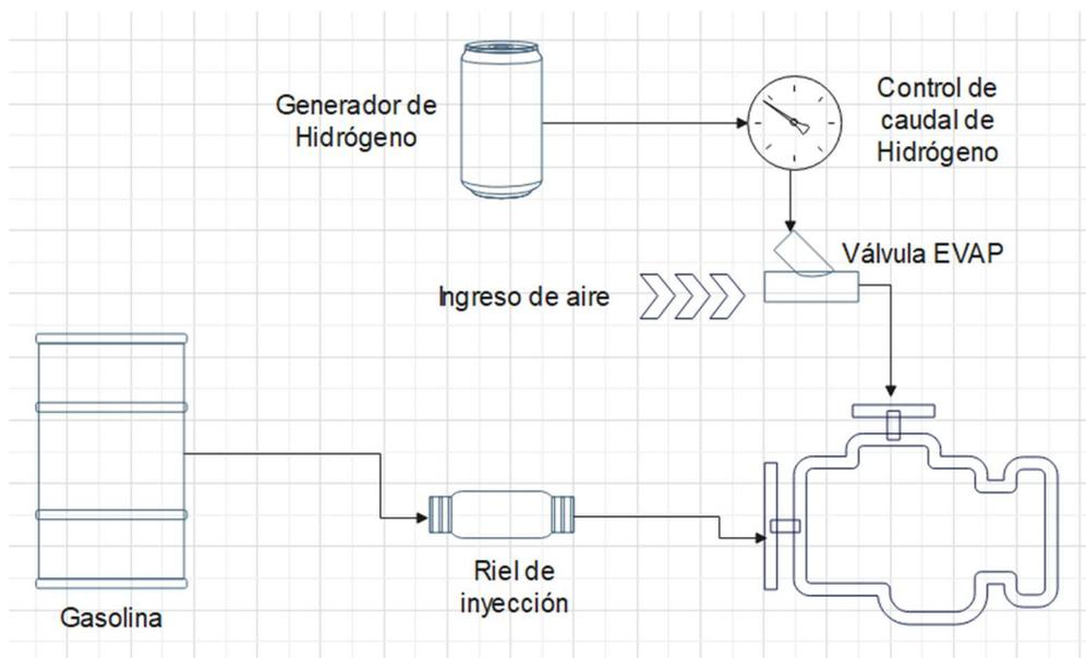
Figure 3 Component Diagram
